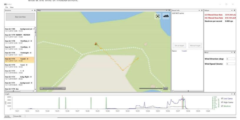
Kolibri software installed on a base station computer. Provides real time processing including ground dose rate calculation and nuclide identification, display, mapping, and data storage.
